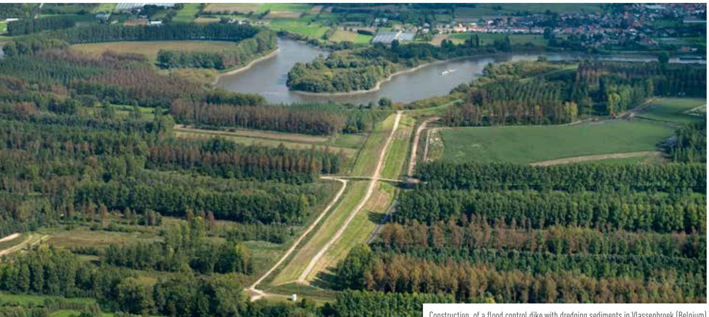
Construction of a flood control dike with dredging sediments in Vlassenbroek (Belgium)
